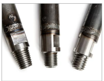
Multi-purpose drill rods are 54mm in diameter and made from high tensile steel used for dynamic sampling and rotary drilling applications. Additional heat treatment is available if required.
